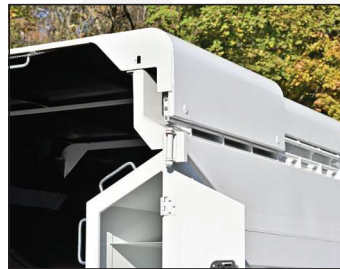
Slide moves on a stainless-steel track
