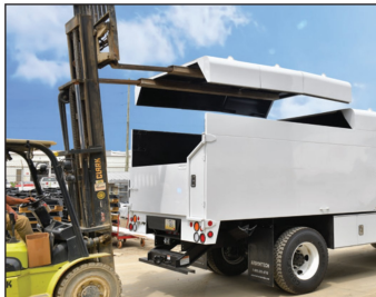
Lift rear sections off
