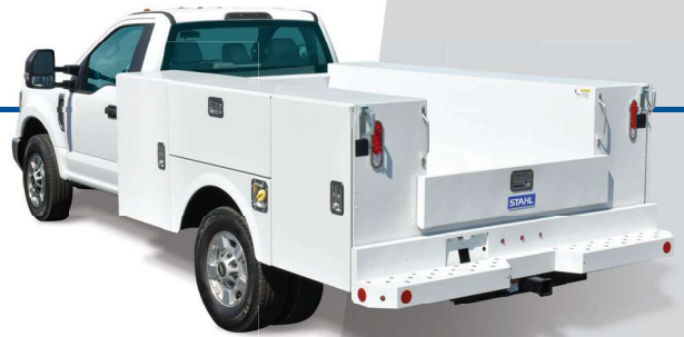
Body pictured with optional Recessed Punched Bumper with surface-mounted LED 3-in-1 Body Light Kit and Aluminum Fuel Fill
