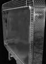
No rear Beams. You can get the unit closer to the cab than a normal CR.
